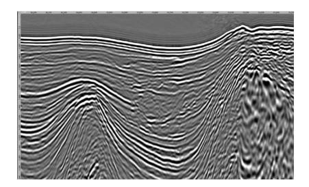
Images on the left show the effect that modern processing and imaging can have on seismic data. Both images were created from the same input data; the DUG result is on the bottom. The hugely increased fidelity allows geoscientists to more accurately evaluate the prospect of hydrocarbons. This kind of processing is necessary for every dataset.
